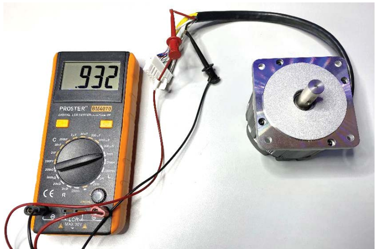
This motor has L_{L-L} = 932 \mu\text{H} line to line inductance (LCR meter leads may also have inductance, use autozero function if available )
