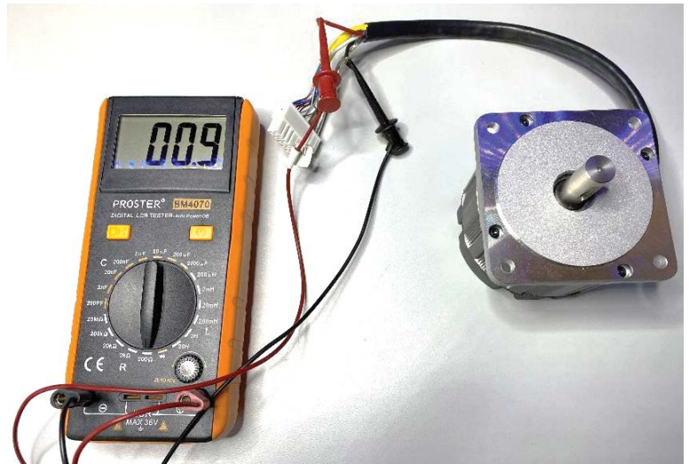
This motor has R_{L-L} = 800 \text{ m}\Omega line to line resistance (100 mΩ due to LCR meter leads)
